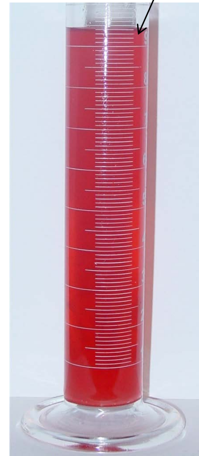
6 hours no agitation, 58% water removed, 42% emulsified 94 ml
